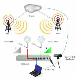
WabMAX continuously monitors the status of each radio-device (i.e. operational or not), the device's wireless performance and its coverage availability. If the combined results are below a predefined threshold for a CPEradio, WabMAX switches the traffic to the next best-available network, while actively updating the network elements about the change. The network handover is transparent to the end-user.
